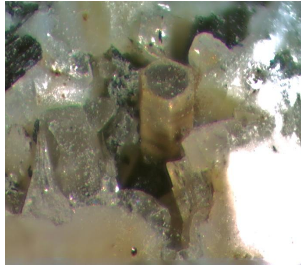
Fig. 1 Synchysite crystal from the Blue Dike Field of view is about 2 millimeters.
