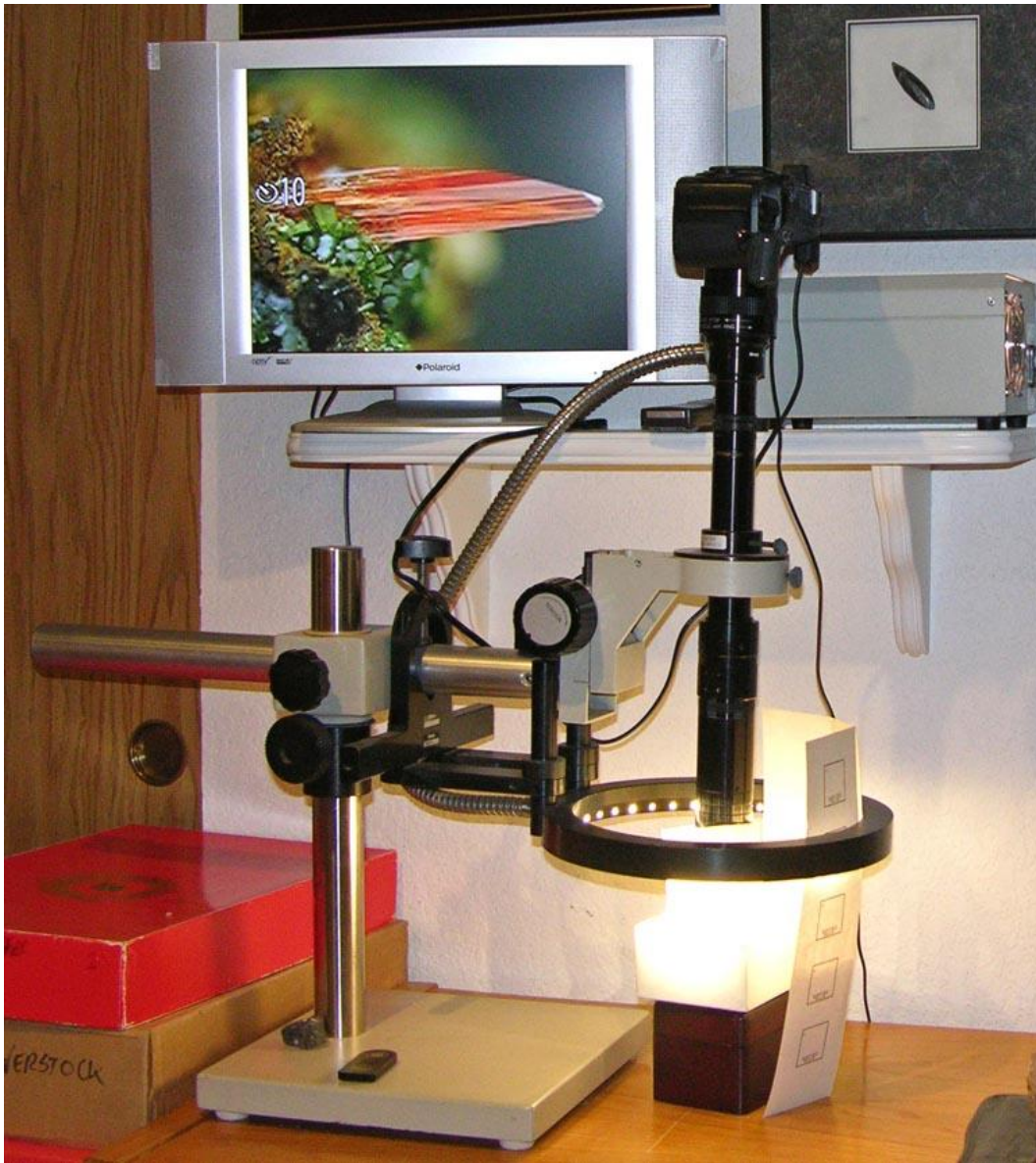
Figure 7: A Micro Mineral Photography setup centered on an Optem Zoom 125C micro inspection lens featuring an 8" diameter fiber optic ring light and a Nikon Coolpix 8400 camera with real-time preview and cordless remote control capabilities.
