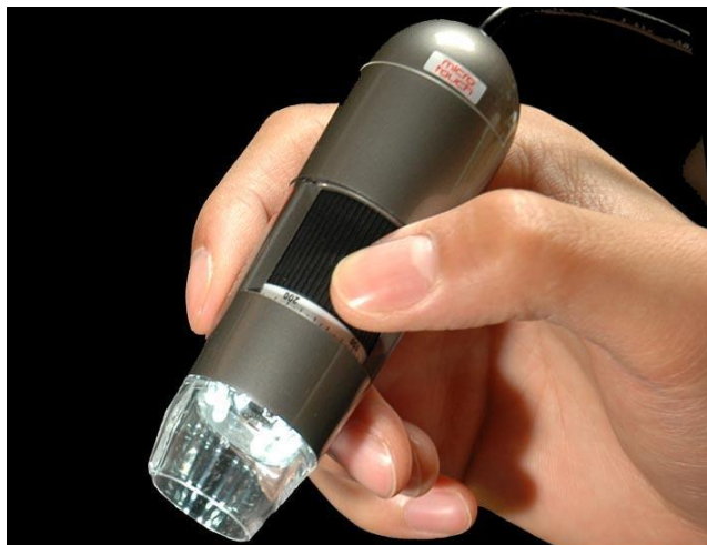
Figure 2: The Dino-Lite, an inexpensive digital microscope (Sunrise Dino, 2011)
