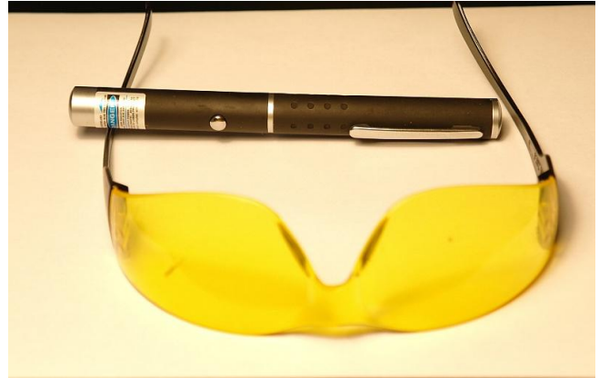
Fig. 2 A 405nm laser penlight and yellow safety glasses
