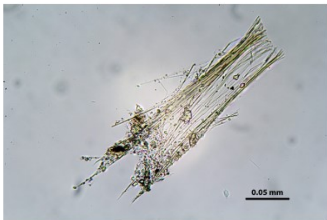
Thomsonite fibers in plane polarized light. Mounting medium is n_D = 1.528 . 250X. Photo by Julian Gray.
