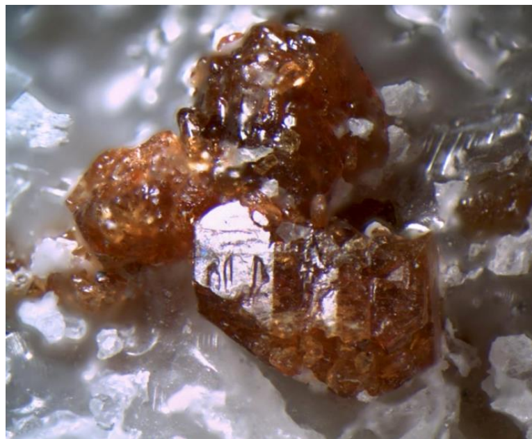
Fig. 3. Hydroxyllellestadite. Twinned monoclinic crystals about a vertical plane perpendicular to the page. Notice the hexagonal shape of the individual nearest the center. (4 mm FS)
